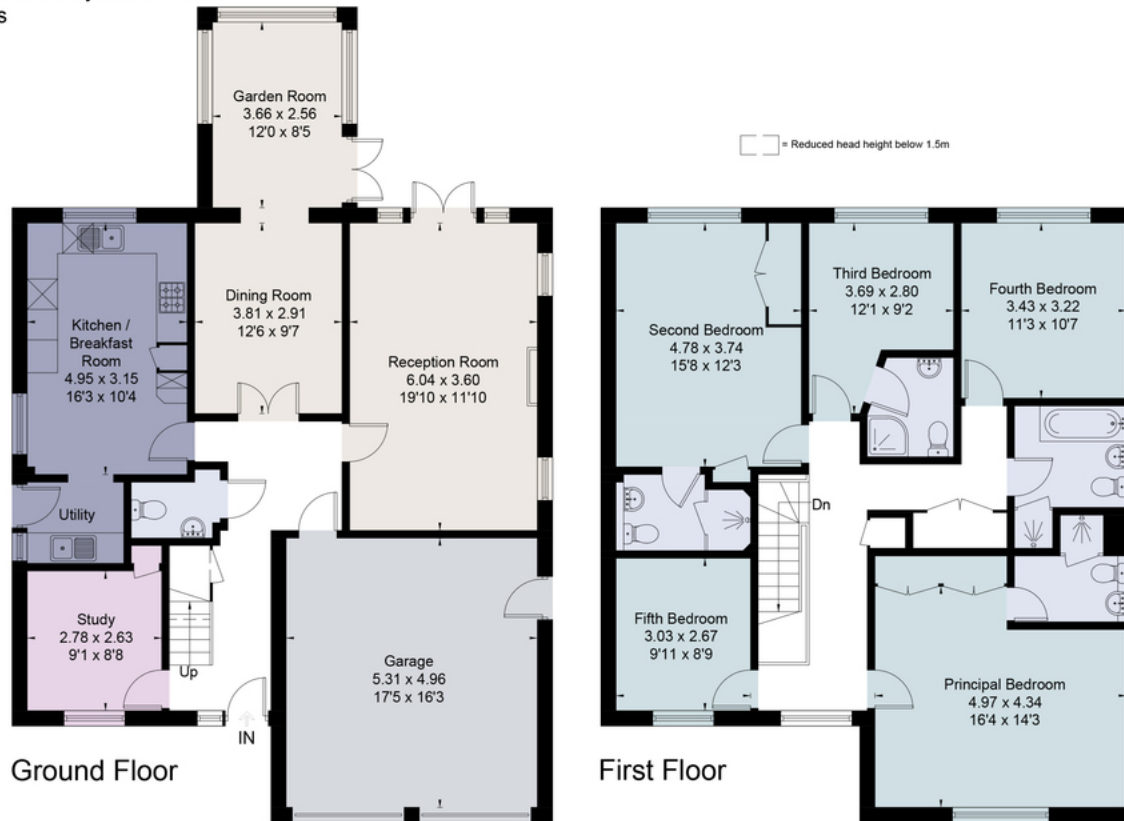
Surveyed and drawn in accordance with the International Property Measurement Standards (IPMS 2: Residential) fourwalls-group.com 297010
