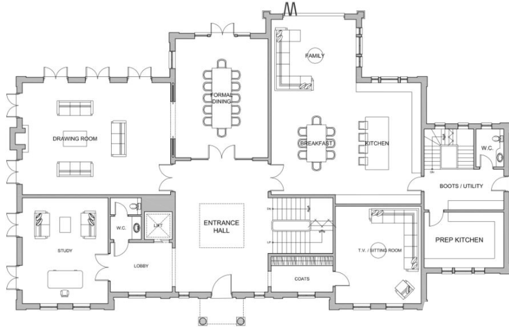
GROUND FLOOR PLAN G.E.A. - 487 m 2 (5,242 ft 2 ) G.I.A. - 446 m 2 (4,803 ft 2 )
