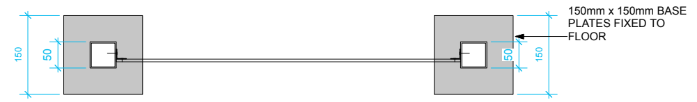
7 Plan through glass Scale: 1:5
